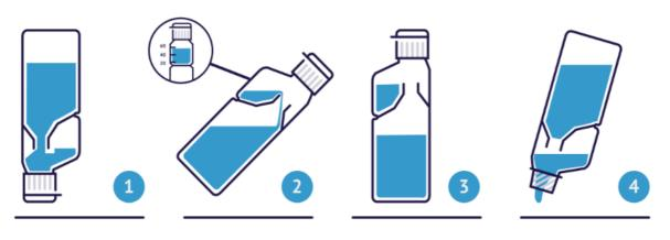
Turn the bottle upside down which will fill the dosing chamber.
